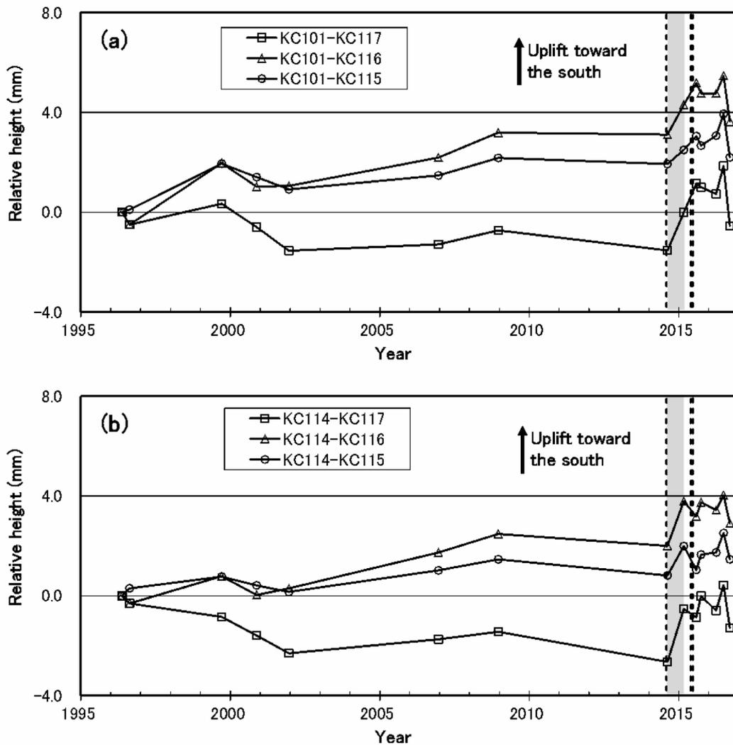
**Fig. 4.** (a) Secular changes of relative heights of benchmark KC101 referring to benchmarks KC117 (open squares), KC116 (open triangles) and KC115 (open circles), respectively, since May 1996. Gray shaded zones denote the period between August 2014 and March 2015 surveys. The three vertical broken lines indicate the timing of the 3 August 2014, the 29 May 2015 and the 18 June 2015 eruptions. (b) Similar to (a) but for the secular changes of relative heights of benchmark KC114.
