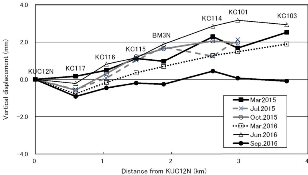
**Fig. 3.** Cumulative vertical displacements of the benchmarks in Kuchierabujima Volcano since the August 2014 survey referring to benchmark KUC12N, which is located at the northern end of the leveling route.
