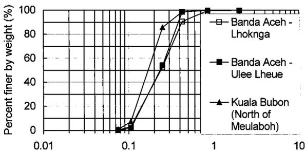
Fig. 6 Grain size distribution curve of sand samples collected at Banda Ache and Meulaboh
