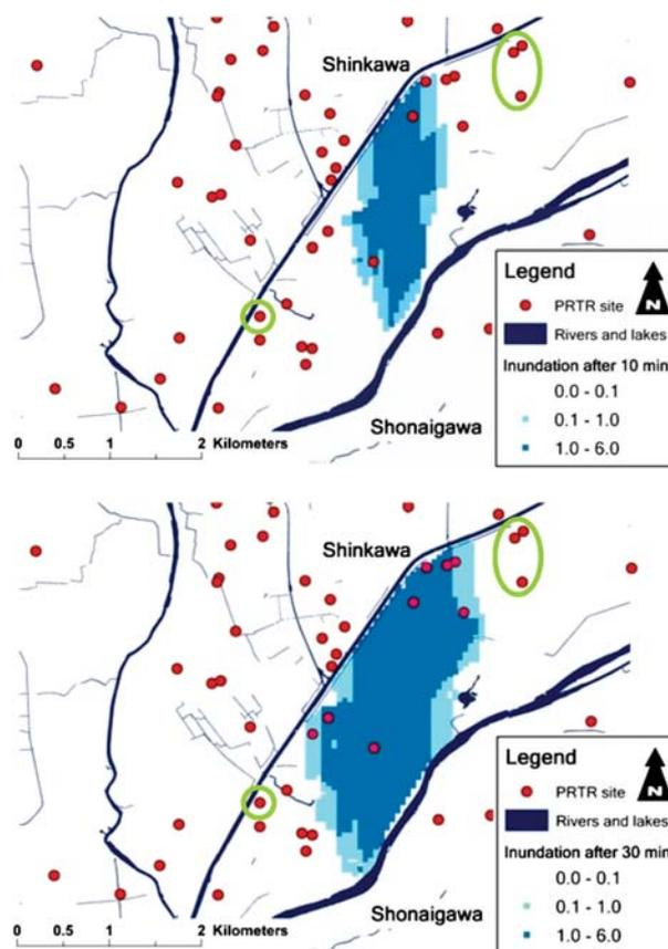
Fig. 4 The marked PRTR-facilities had more than one-hour time for preparation and were inundated with less than one meter height. Compare with Fig. 1.
