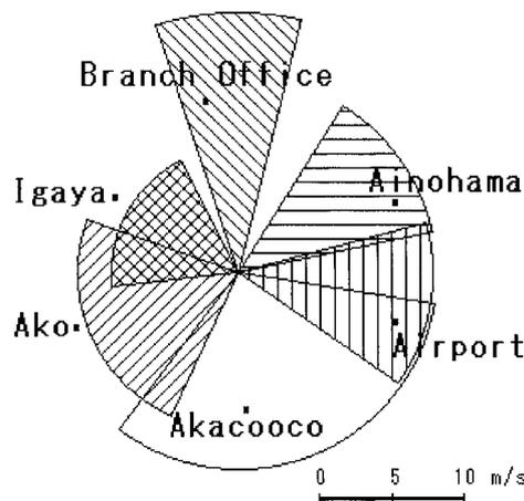
Fig. 5 Graph of Table 2. The radius and angle of each sector respectively show the average wind velocity and wind direction range values obtained from the average value +/- the standard deviation. The center represents the crater of the volcano. The relative location of each station from the crater is shown by a closed square.
