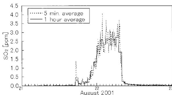
Fig. 3 Comparison of five-minute and one-hour  $\text{SO}_2$  concentration values.
