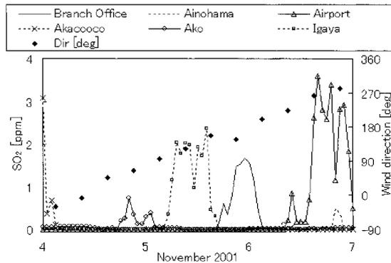
Fig. 7 Temporal variations in the one-hour  $\text{SO}_2$  concentration values at six stations (left) and 925 hPa wind directions at Hachijyojima (right) from 4 to 6 November 2001. The first two pairs of wind directions are the values for -360 degrees subtracted from the raw data to maintain varying wind direction continuity.
