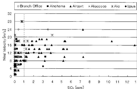
Fig. 6 Scatter diagram of the wind velocity and SO<sub>2</sub> concentration at each station at wind observation time for a leeward direction within 10 degrees.
