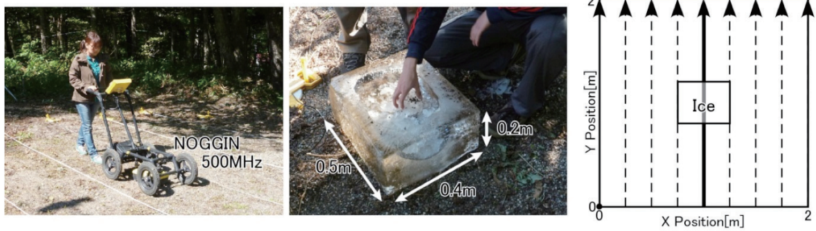
Fig. 2. GPR survey of the buried ice and the survey lines.
