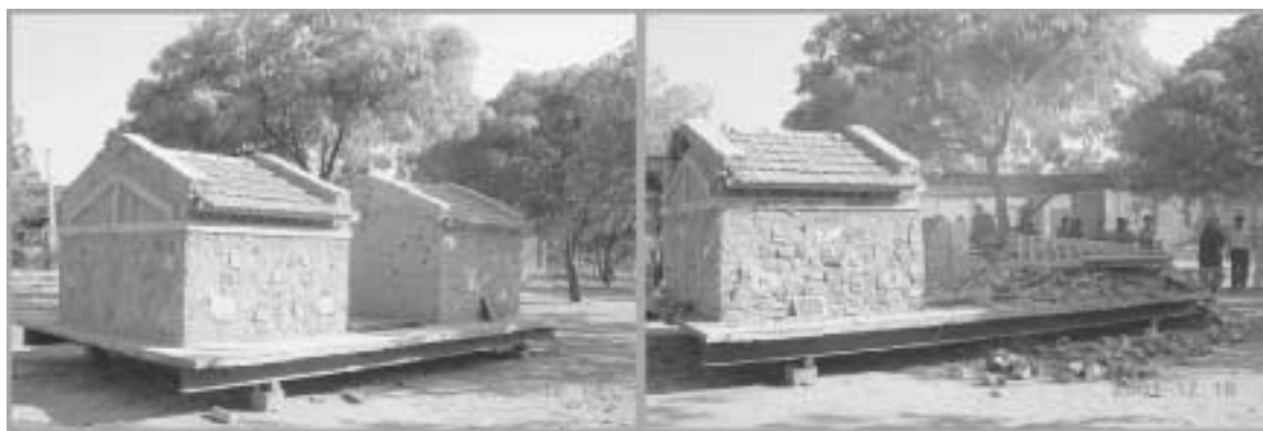
Fig. 6 Shake table demonstration tests. Normal construction (model right), improved construction with retrofitting (model left), Photo : left before testing, right : after testing.
